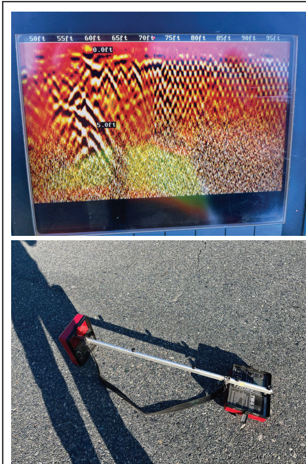
Fig. 1: All of the equipment was used in an octagonal-grid pattern across the entire area of investigation (AOI). Sample GPR data set shown.
