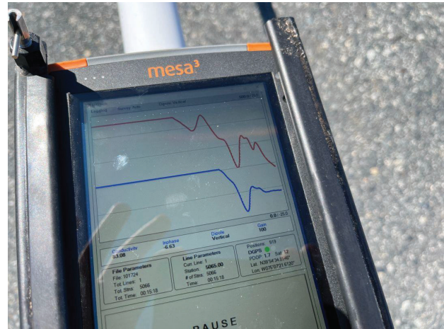
Fig. 2: The AO I was investigated using the Geonics EM31-MK2 ground conductivity meter. Sample images of data sets shown.
